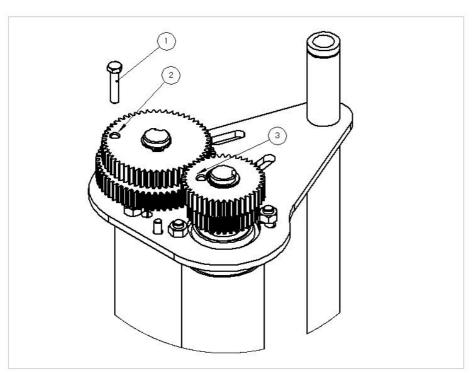
If the bolt (1) is fitted in position 2, the top set of gears provide the stretch (70%).
