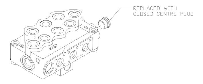
If you are likely to change frequently between open and closed centered hydraulic systems and special plug incorporating a tap can be ordered. (Part No. 1008050- closed center tap plug). This is fitted in the same position on the valve.
